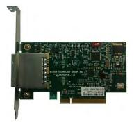
For low profile case applications, you may need to change the mounting bracket to the low profile bracket that shipped with your system. This is done by removing the screws that hold the card to the bracket. Be sure you are using proper ESD procedures when completing this action.
