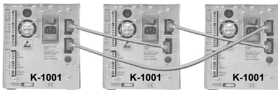
Fig. 24 Connection scheme of three HPLC pumps K-1001
