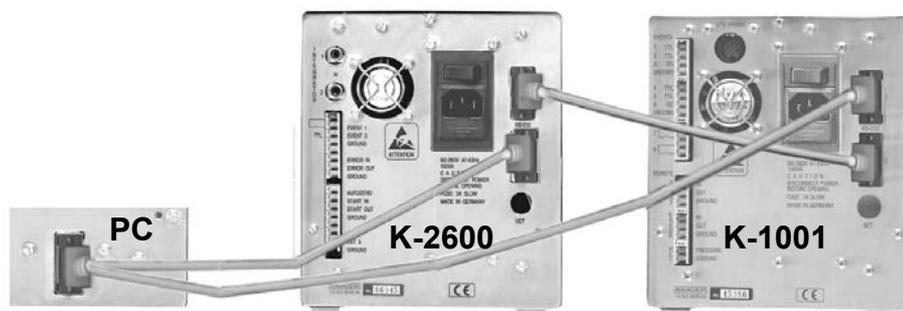
Fig. 25 Connection scheme of a HPLC pump K-1001 with PC and other instruments
