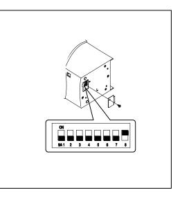
Note: Always change DIP switch settings only when the printer is turned off. Change made with the power on have no effect and then on again.
