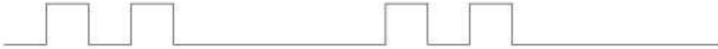
Example of a 2-impulse train. In the event of an impulse, the ON/OFF Led lights up.
