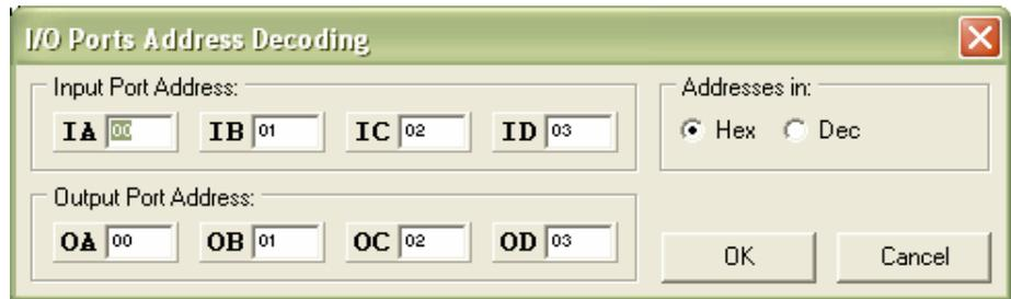
Fig. 85: Port addresses can be modified in the "I/O Ports Address Decoding" dialog window.
