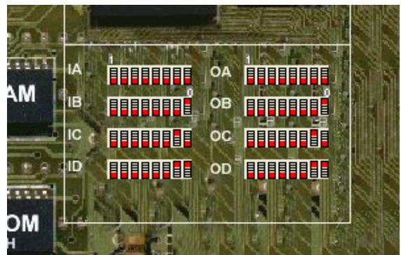
Fig. 86: Port addresses can be modified by a mouse click on the simulated 'on board' dip switches.
