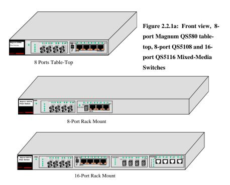
. Mixed-media combination modules (4-port modules with three fiber ports and one twisted-pair port) are supported in all of the Quad-Series Fiber Switch models. All quad-module manual-selection switches and LED's are located on the front panel, with the IEC standard AC power connector (and a manual ON - OFF power switch) located at the rear. Fan-driven cooling air flows left to right.
