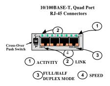
unshielded twisted pair (UTP) and shielded twisted pair (STP) cable connections.
