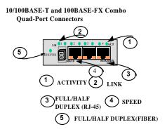
functions as a fiber optic transceiver to support 100BASE-FX network segments. When installed in a Quad-Series Fiber Switch, it supports fiber cable distances up the IEEE-standard 100Mbps distance limits, i.e., typically 2km at full-duplex and 412m at half-duplex. The factory default setting is for full-duplex operation, and a jumper on the module must be moved to select half-duplex. (See Section 3.4).
