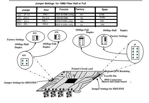
Figure 3.7 10Mbps Fiber ports internal jumper settings.
