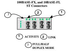
Each port has an Activity (ACT) LED indicating packets being received, a Link (LK) LED that indicates proper connectivity with the remote device when lit, and a FDX/HDX LED to indicate full-duplex mode when lit (or half-duplex when off). Lettering on the front of the module identifies it as "100 FX" to avoid confusion with other similar-looking 10 Mb fiber QPMs.
