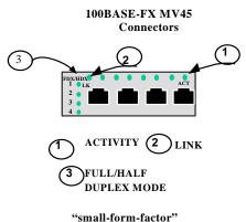
The small size of the VF-45, about the same as an RJ-45 port, reduces the size of wiring panels in wiring closets while providing the advantage of "future-proof" fiber optic technology.
