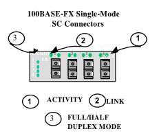
supports single-mode fiber cable lengths of as much as 25+ Km (see Power Budget, Section 4.5)
