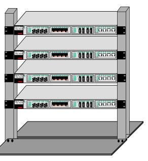
Fig 3.8 Multiple Magnum QS5116 units rack-mounted in a 23" frame
