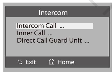
1. **Intercom Call:** User in one apartment can call other apartments in the system. the code list will be created automatically by the system. Touch a code number you require on the screen, then touch ☎ icon to dial. (Note: Touch ☎ icon again to redial. 2.The DIP switch codes of each monitor must be set using the **Physical Code Method**.)
