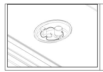
To seal the scale a lead-wire seal can be used as shown below. The base has a metal pin that protrudes through the cover. The security seal may be threaded through this metal pin, making it impossible to remove the cover without damaging either the security seal or the enclosure.
