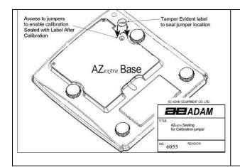
The calibration of the AZextra scale is accomplished by removing the label at the base of the scale which covers a hole through which the PCB can be accessed. If your scale is not provided with this hole, you need to break the security seals and remove the top cover to gain access to the circuit boards inside. See the figure on the security seal below.
