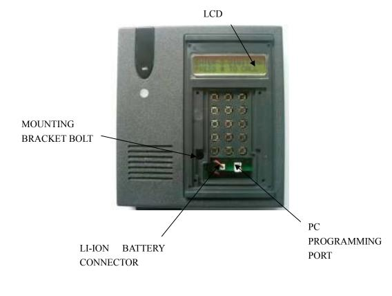
Mounting of Caller Unit INSERT RIVERTS INTO HOLES (FOR CONCRETE WALL ONLY)
