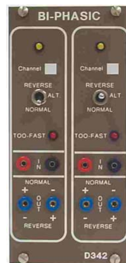
The D342 dual bistim module allows stimulus polarity to be alternated
