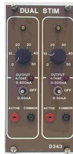
The D343 constant current dual channel stimulator module
