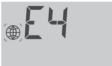
Fig.: Example for a blinking code sequence for Internet - Fault 4
