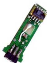
111 9590 DCC-1 digital capacitive cell- silicone based
