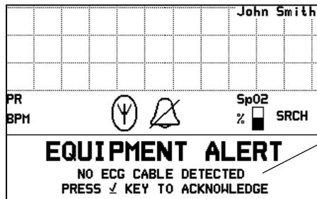
The monitor has detected that the ECG cable has been disconnected from the monitor.
