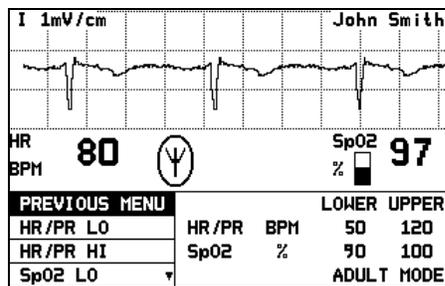
Alarm limits can be adjusted for HR/PR and SpO<sub>2</sub>.
