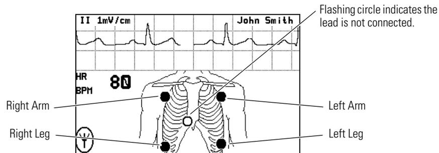
If the monitor detects that some lead wires are not properly connected, the monitor displays a chest diagram and indicates which leads are disconnected.
