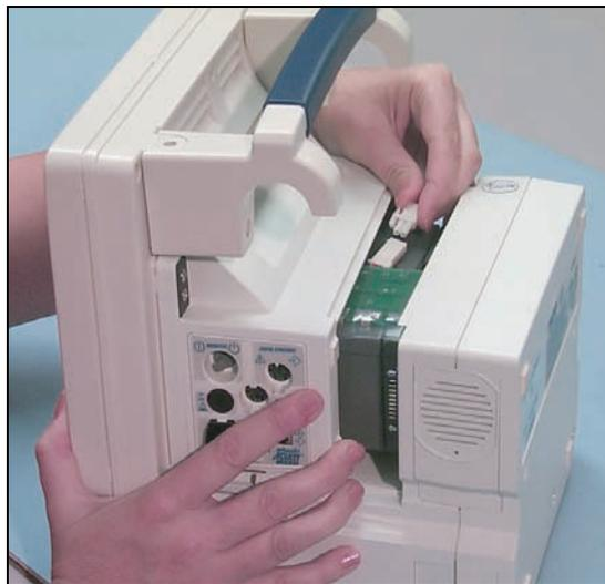
4. Continue to slide the monitor forward until it can be completely separated from the Expansion Module.
