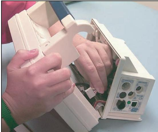
6. Spread the casing open to an angle of about 45-60 degrees.
