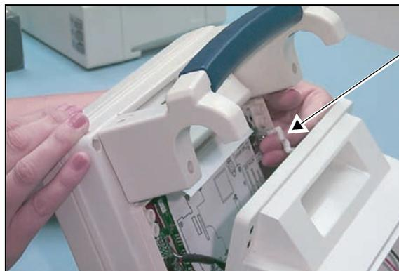
Disconnect tubing from pressure transducer
