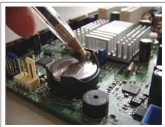
The horizontal carrier has a spring located underneath the battery which will eject the button cell once the clip is pushed clear off the battery. Apply pressure to the clip with a device such as a pen, or by using the tip of your finger.
