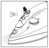
**Note:** For Spray and Shot of Steam functions to operate, the water tank must be at least one-quarter full. If these features stop working, stand the iron on its heel and fill the water tank.
