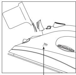
Do not fill the iron above the MAX mark indicated on the side of the iron.
