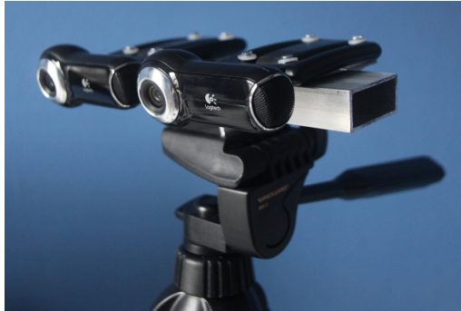
Figure 4: Tripod with cameras in horizontal capture position
