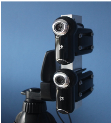
Figure 5: Tripod with cameras in vertical capture position
