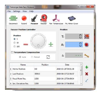
The Focuser Control tab allows the fine-positioning of the Camera Focuser. The Focuser position is given in steps - one step corresponds to 1/40000<sup>th</sup> of an inch. The control tab works similarly to the rotator controller but offers some additional features such as temperature compensation and a deviation display. The focuser is mechanically limited in its movement and thus offers two optical limit switches on both ends of the slew axis.
