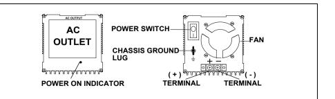
CAUTION: DO NOT REVERSE INPUT. USE RED BATTERY CORD TO CONNECT (+) OF A DC BATTERY TO (+) TERMINAL. AND THEN, USE BLACK BATTERY CORD TO CONNECT (-) BATTERY TO (-) TERMINAL.
