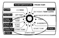
tive stages are adjusted by the same amount. The bandwidth can be adjusted from  $0.5^{\circ}F$  to  $20.0^{\circ}F$  ( $0.3^{\circ}C$  and  $11.1^{\circ}C$ ).
