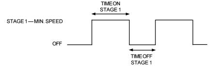
During time on, the Stage 1 fans run at Stage 1 minimum speed. The Stage 1 Pilot Light turns on. During time off, the Stage 1 fans do not run. The Stage 1 Pilot Light turns off. The Stage 1 minimum speed can also be defined by a speed curve (see below).
