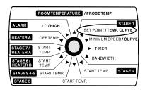
The temperature set point is the target room temperature. It can be adjusted between -40.0°F and 99.9°F (-40.0°C and 37.7°C).
