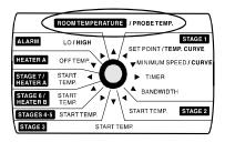
The readout can display values from -40.0°F to 120°F (-40.0°C to 48.9°C). When the temperature drops below -9.9 degrees, the negative sign is displayed separately, alternating with the numerical value.
