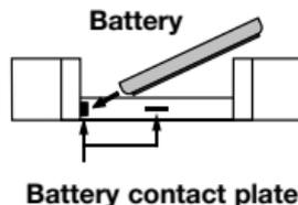
1. Open the sensor battery lid with a coin by turning counterclockwise.
