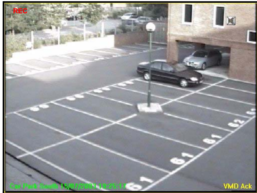
Figure 2-2: Text labels displayed in a Live Camera View
