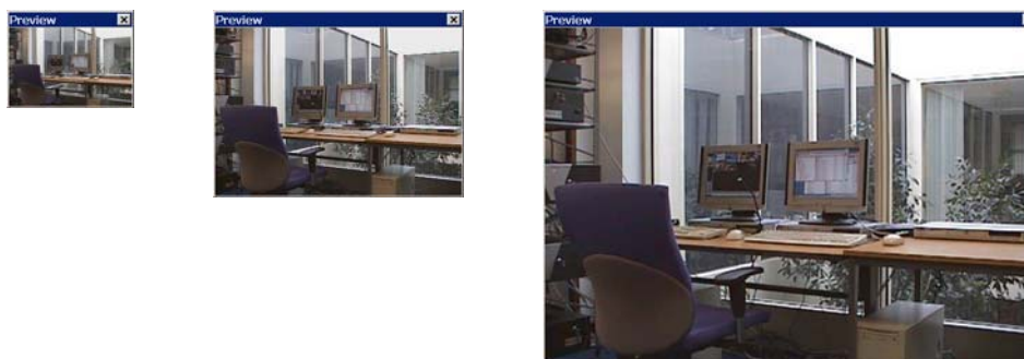
Figure 5-6: Previews of three resolutions for an IP camera. (Left: 176x112 Centre:352x240 Right: 704x480)
