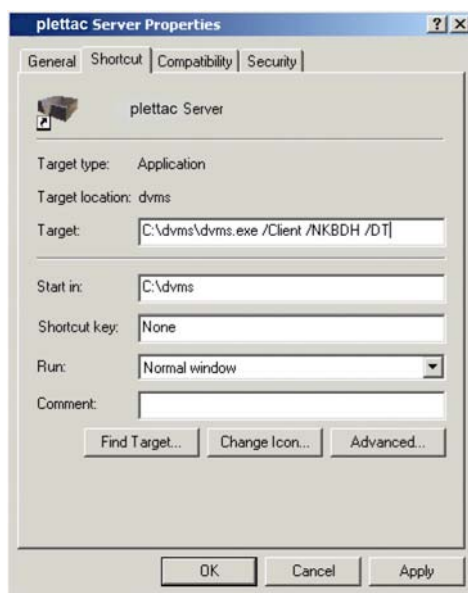
Figure G-2: Setting Run-Time Parameters in the Properties dialog
