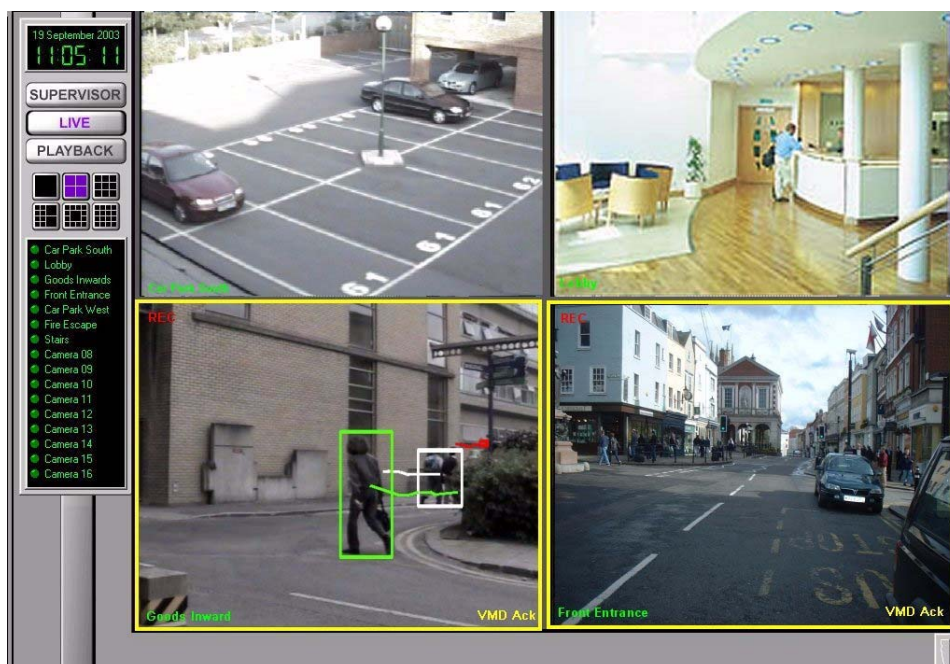
Figure 12-8: SVMD Output on Live Display of plettac Server's GUI
