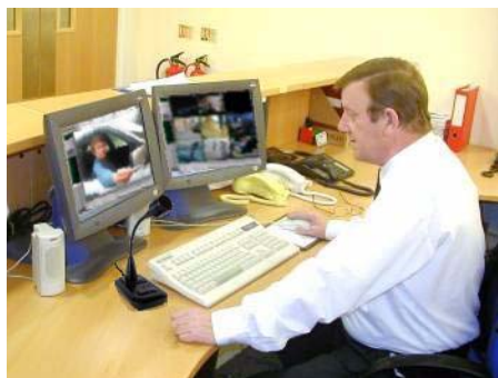
Figure 12-12: Two-way conversation using Bi-directional Audio
