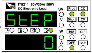
2) Press very key to enter TYPE setting. Use the knob to switch the working mode, CC mode, CV mode, CR mode.
