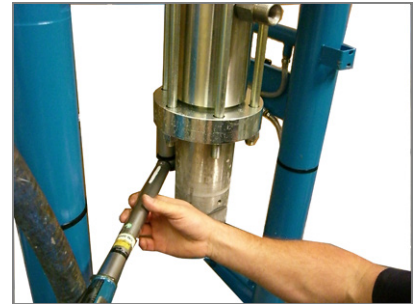
Fig. 20: Unscrew the nuts on the threaded bolts
