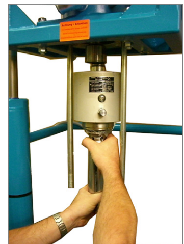
Fig. 23: Remove the HP-head and the dual piston from the coupling
