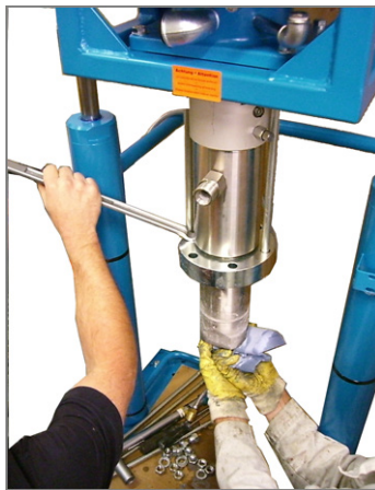
Fig. 21: Pry the pressure cylinder from the spring housing
