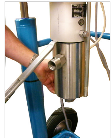
Fig. 22: Pry the spring housing from the HP-head
