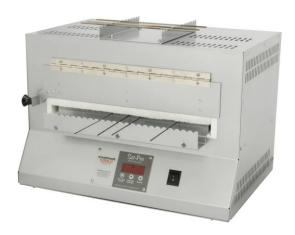
Lift the door of the Fishbone and place your glass laden mandrel on the mandrel rest as shown. Once you have loaded the beaded mandrel, close the door. Repeat this procedure for each bead you make. It should be noted that except for the loading and unloading of individual beaded mandrels, the door on the Fishbone should remain closed. So, closed at all times except when loading or unloading.
