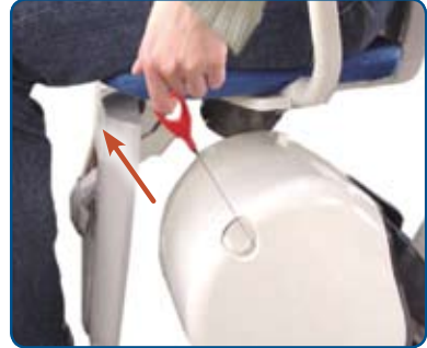
Fig. 2/6: Making the lift descend in an emergency
