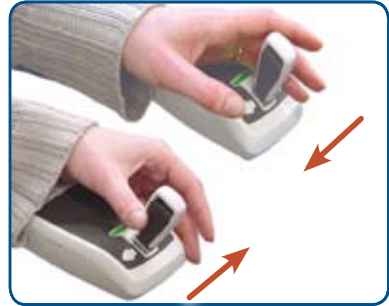
Fig. 2/18: Hold the joystick in the required direction.
