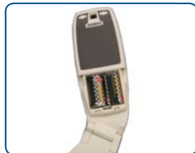
Fig. 4/2: Armrest control batteries.
