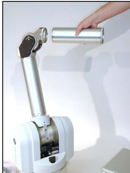
Figure 7 - Separating the Outer Link
