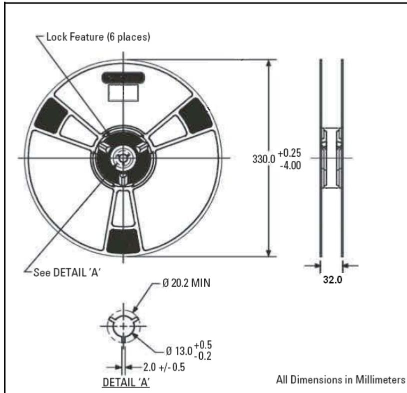
Figure 8.2 Reel Diagram
