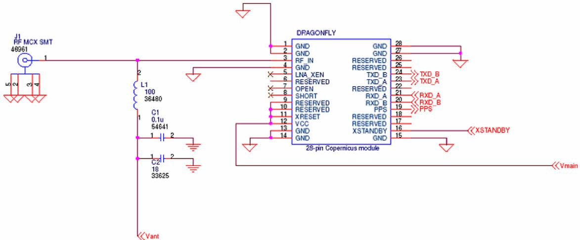
Figure 5.4 Application Drawing: Active antenna - No Antenna Status
