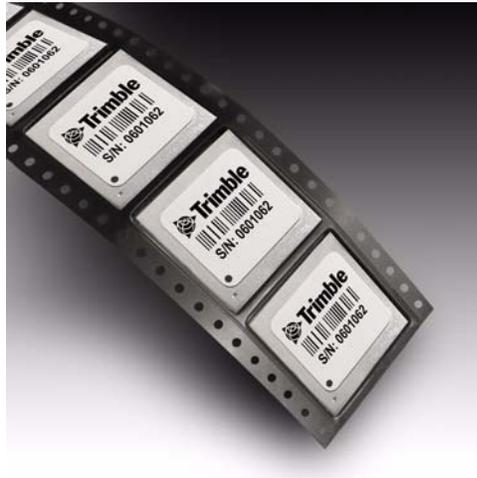
Figure 8.1 Copernicus GPS Receiver Packaged in Tape
