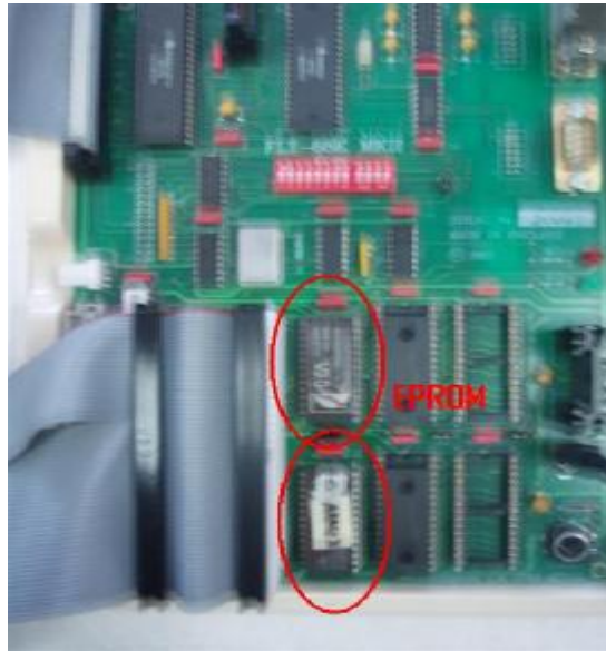
Figure 17: Replace the EPROM from the 68000 microprocessor board
