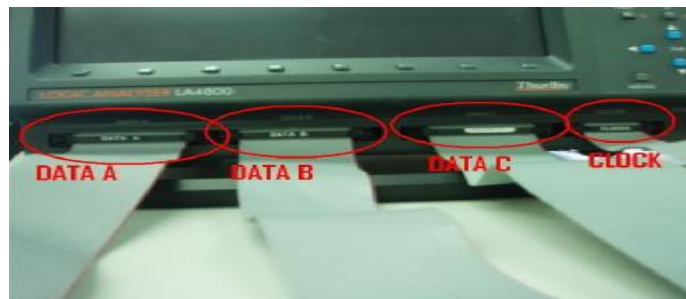
Figure 3: Connection to the Logic Analyser
