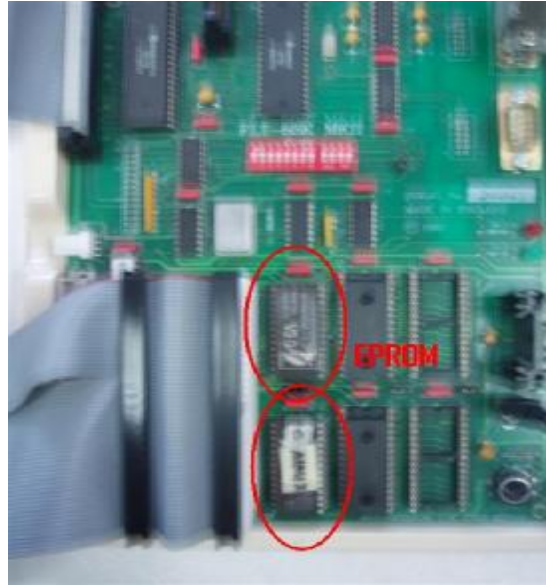
Figure 3.12 Replace the EPROM from the 68000 microprocessor board
