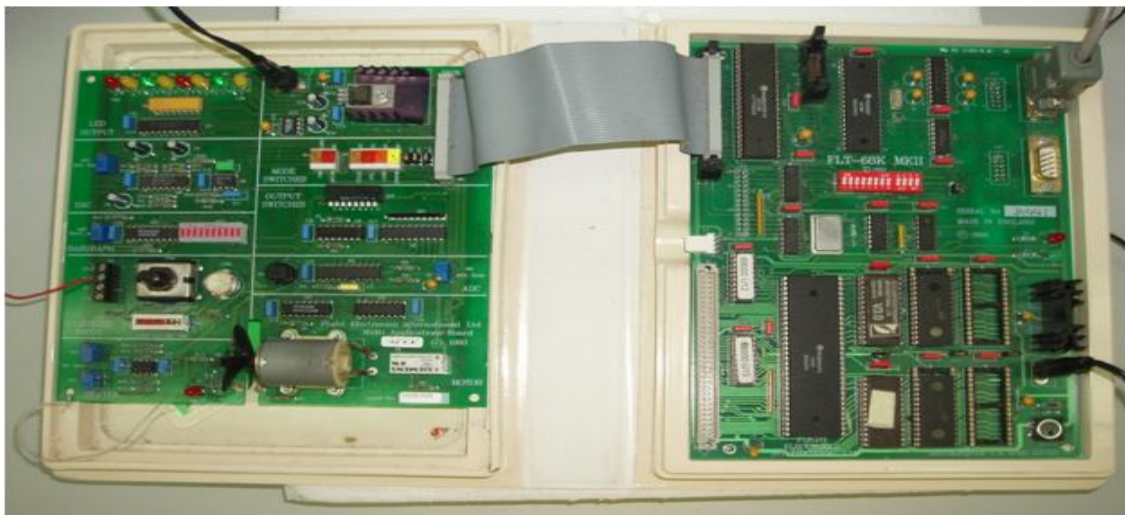
Figure 2.12 Application Board (Left Side) and 68000 Microprocessor Board (Right Side)
