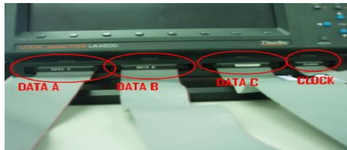
Figure 3: Connection to the Logic Analyser
