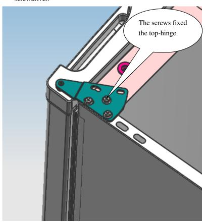
3. Replace the top-hinge and the door limit block and the door bearing bush to the other side
