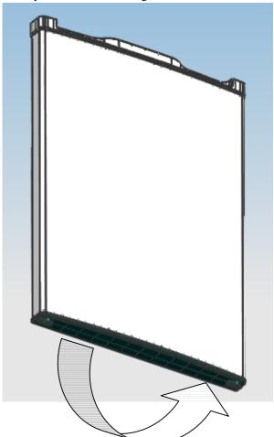
4. Disassemble the screws fixed the bottom-hinge with cross-slot screwdriver and replace the hinge to the other side then fix it with screws  $_{\circ}$
