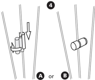
4. There are two spoke magnet options. **You only need to install one of them.** Check which of the magnets fits the spoke of your bike best. (A) One is installed by rotating it around the spoke before putting the metal cover on, another (B) by tightening the screw. The magnet must be facing the speed sensor.
