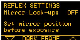
**IMPORTANT WARNING: Mirror lockup is suitable for DSLR cameras allowing the mirror raising. The same setting (either ON or OFF) MUST be applied both to the SmartGuider 2 AND the Reflex at the same time, otherwise erratic behavior may result.**
