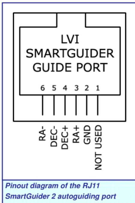
The SmartGuider 2 camera comes with an “open collector” autoguider port, fully compliant with the ST4 standard. This means it can be plugged straight into all most popular equatorial mounts having such an autoguider port.
