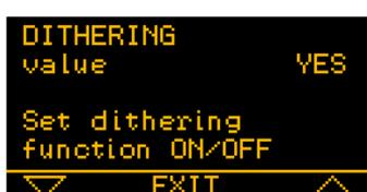
Next, with **DITHER** we get to the **DITHERING** menu. If turned on (**YES**), the SmartGuider 2 will apply a **very small** displacement to the field of view along both axes after each exposure taken with the reflex camera controlled by the MGA. With dithering off (**NO** in the menu), the guide star will always be staying in the same position where it originally was when autoguiding started.
