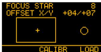
If the star happens to be lying too close to the sensor boundaries (Offset limits:  $X = \pm 82$ ,  $Y = \pm 46$ ), you may want to move it toward the center by **CAREFULLY** nudging the mount with the drive keypad at guiding rate.
