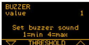
You can adjust both the brightness and the buzzer volume with the two triangular keys on the control paddle: four levels are available, from **1** (minimum) to **4** (maximum). **EXIT** takes you back to the basic settings screen.
