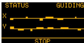
The two graphs allow real-time monitoring of guiding corrections issued to the mount. You can stop the autoguiding process by pressing **STOP** at any time, while **EXIT** will take you back to the **MENU BASIC**.
