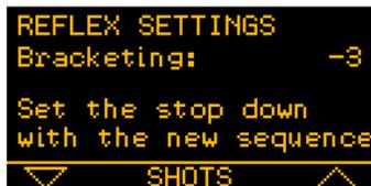
Then we have the **BRACKETING** menu. This feature allows to set up an additional imaging sequence, whose exposure time is calculated by applying the stop-down setting to the main sequence’s value. The stop-down can take four values: **OFF** (bracketing off), **-1** (-1 stop, i.e.
