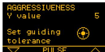
With the two arrow-shaped buttons (**UP** and **DOWN**) on the camera pad, you can adjust the aggressiveness along the **X axis** (upper left screen) and along the **Y axis** (upper right screen) of the detector.
