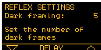
Next, choosing **DARK FRAME** opens the dark frame configuration screen. Dark frames will have to be subtracted from raw shots during the post-processing phase: this helps in cutting down thermal noise which is present especially in long-exposure images. With the two arrow buttons, we can select from **1** up to **10** dark frames, whose exposure length will be the same as that of the main sequence.
