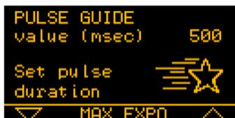
By choosing **PULSE**, we get to the screen where we can set the length of the guiding corrections the SmartGuider 2 sends to the mount. These corrections are sent as pulses of given duration (in milliseconds) which can be adjusted via the two arrow-shaped buttons.
