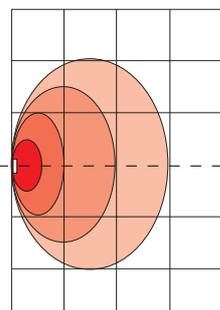
Noise level diagram at 6 bar air pressure.
