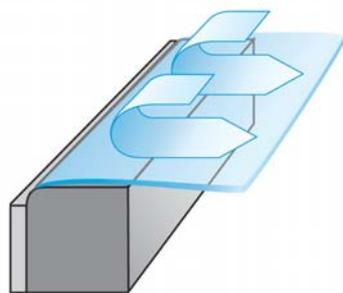
The air blade exiting through the side slot follows the radiused profile and leaves the body with an angle of 90° from the original direction, as shown by the drawing. This remarkable feature, based on the Coanda effect, makes it possible to have the air outlet orifice in a totally protected position, which is very interesting as for instance in those cases where products oscillating on a chain conveyor can damage conventional air blowers.
