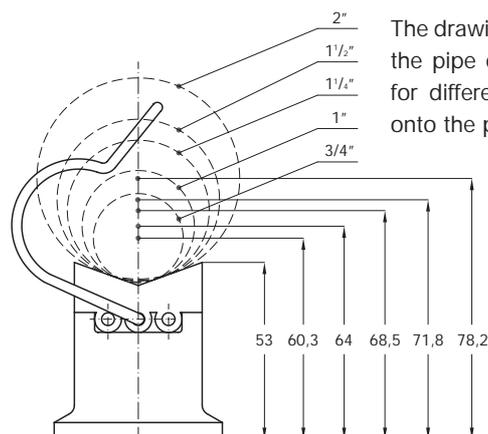
The drawing shows the distances of the pipe center axis from the wall, for different pipe sizes assembled onto the pipe holder.
