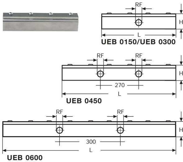
UEB blowers produce a laminar jet of compressed air, with high efficiency and limited noise level. Their unique design provides an air stream exiting from a protected position, and changing direction because of adhesion to a radiused profile due to the Coanda effect. Their design allows for remarkable advantages:
