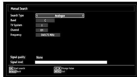
After selecting search type as **Manual Channel scan**, you can use **Up** or **Down** button to highlight an item and then press **Left** or **Right** button to set an option.
