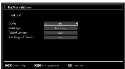
3. By pressing **Left** or **Right** button, select the **country** you want to set and press **Down** button to highlight the **Search Type** option. Use **Left** or **Right** to set the desired search type. Available search types are Digital and analog, digital only and analog only.
