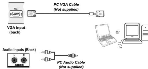
To use a PC, set the monitor output resolution on the PC before connecting it to the television. To display the optimum picture, use the PC setting feature.
