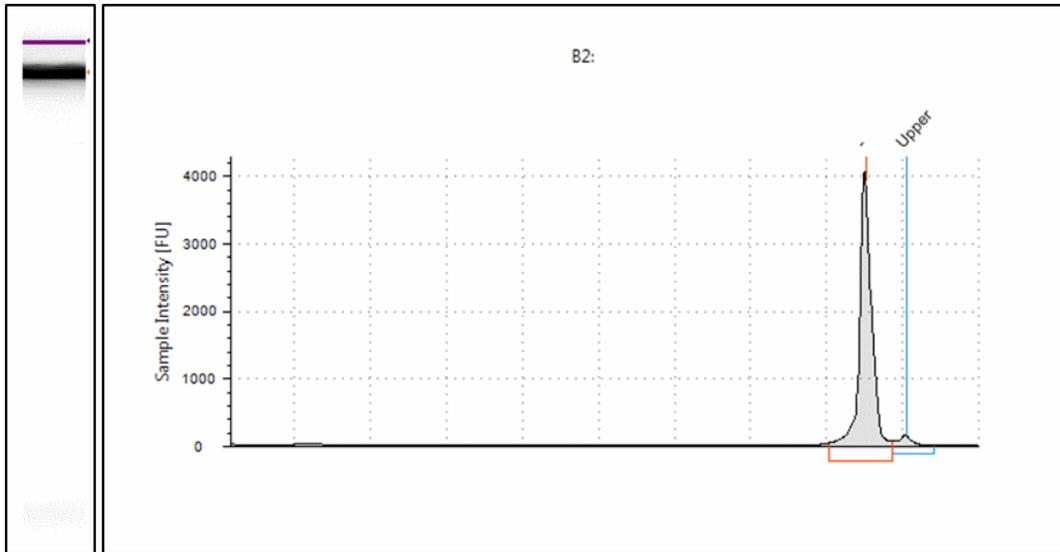
**Figure 14** Example of missing marker peak
