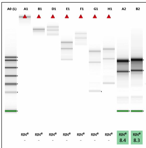
**Figure 30** Example of short migration caused by high salt concentration. Lanes A1- B2 show the same sample in buffers of decreasing salt concentrations, allowing migration further through the gel lane.
