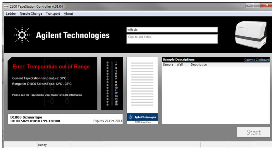
**Figure 3 Error: Temperature out of Range**
