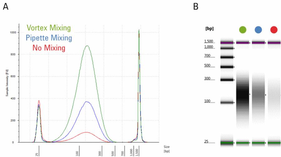
**Figure 7** The electropherogram (A) and the gel image (B) of the ScreenTape mixing tests. In both panels the green trace shows the recommended protocol of vortex mixing using the IKA vortexer and adaptor at 2,000 rpm for 1 minute followed by brief centrifugation. Blue shows results for pipette mixing only. Red shows the effect of no mixing. Images were taken from the Agilent TapeStation Analysis Software
