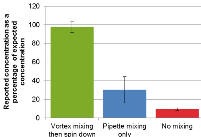
**Figure 8** Chart of reported concentrations for the ScreenTape mixing tests, using the D1000 Assay. Concentrations are expressed as a percentage of the theoretical for the three mixing methods. As above, the green bar represents the recommended protocol of vortex mixing using the IKA vortexer and adaptor at 2,000 rpm for 1 minute followed by brief centrifugation; blue - pipette mixing only; red - no mixing.
