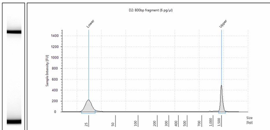
**Figure 17** Example of missing sample peak
