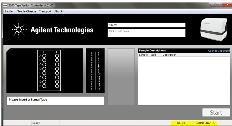
**Figure 33** Controller software indicating a Preventative Maintenance is due. Schedule Preventative Maintenance, do not perform a Needle Change
