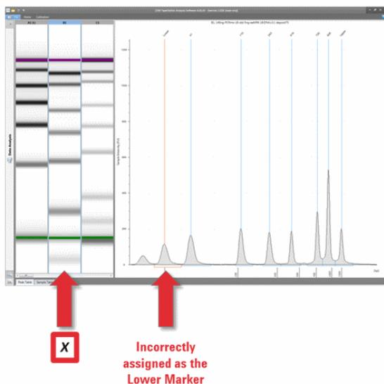
**Figure 15** Identifying the correct lower marker
