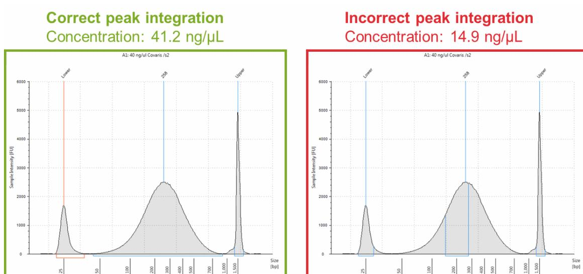
**Figure 10** Example of correct (A) and incorrect (B) sample peak integration, and their effect on reported sample concentration.
