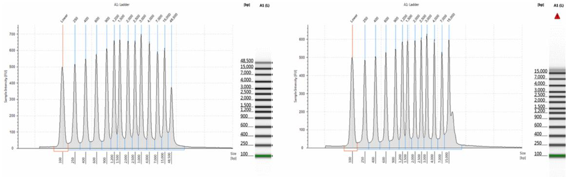
**Figure 13** The effect of shaking the Genomic DNA Ladder. A) Genomic DNA Ladder has been vortex mixed for 5 seconds prior to analysis on the Genomic DNA ScreenTape assay. B) The Genomic DNA Ladder vial was shaken by manually inverting the tube 30 times. Degradation of the top fragment (48,500 bp) is clearly shown.
