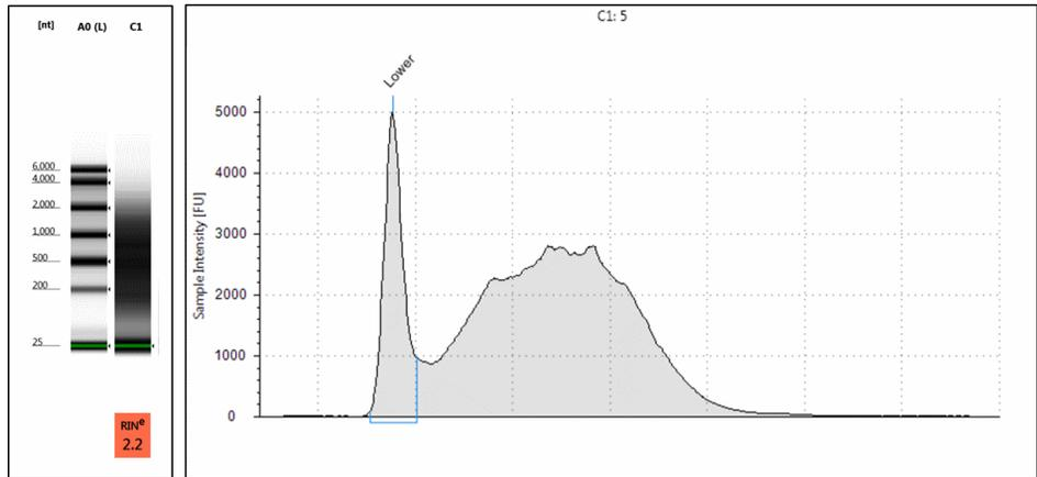
**Figure 25** Example of degraded RNA resulting in missing peak identification.
