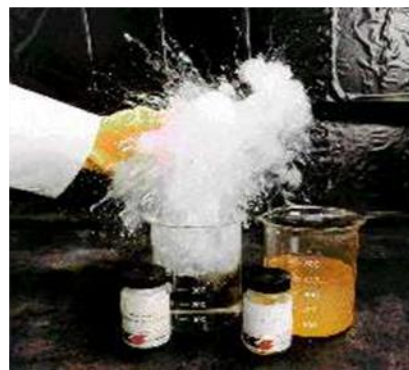
Figure 9 The Explosive Addition of \text{AlCl}_3 to Water
