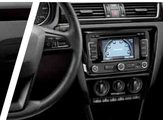
PIANO BLACK DASHBOARD DECORATIVE. Piano Black decorative cover for the radio and climatronic frame. They are attached to the original part. 6JA072525B
