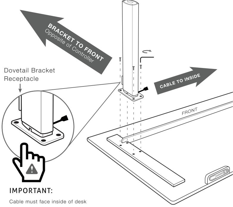
Dovetail bracket receptacle must face front of desk.(opposite of controller)
