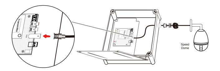
5. Feed RS485 signal cable through cable gland to connect with transmitter.
