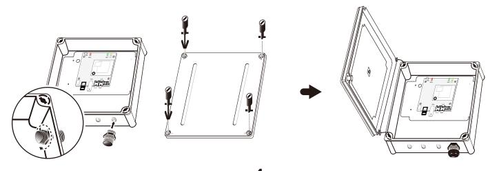
2. Locate transmitter box on the elevator. (Depending situation on bottom or top)
