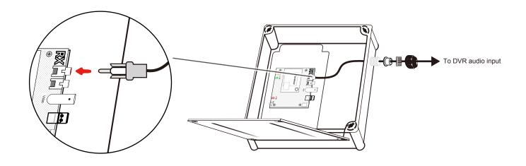
7. Feed power cable through cable gland to connect with Receiver.
