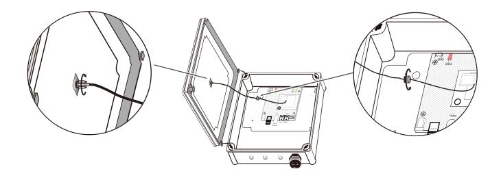
4. Feed video signal cable through cable gland to connect with Receiver.
