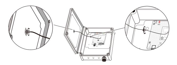
4. Feed video signal cable through cable gland to connect with transmitter.
