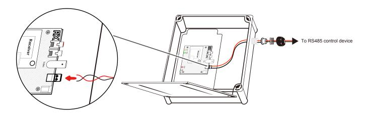
6. Feed audio signal cable through cable gland to connect with Receiver.
