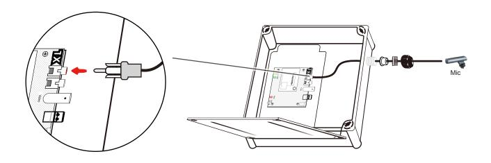
7. Feed power cable through cable gland to connect with transmitter.
