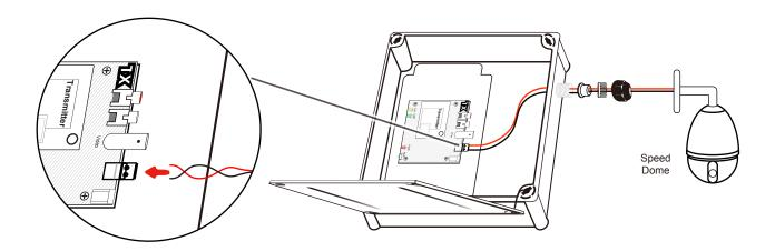
6. Feed audio signal cable through cable gland to connect with transmitter.
