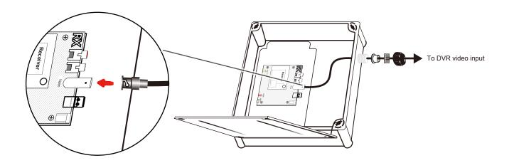
5. Feed RS485 signal cable through cable gland to connect with Receiver.
