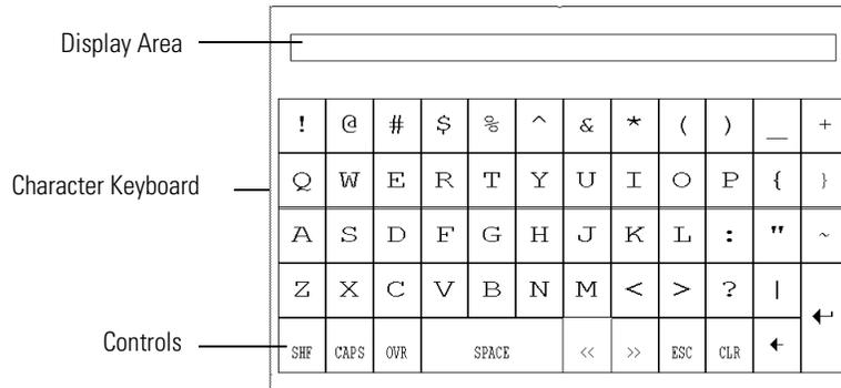
Select characters by touching the Character Keyboard on the screen. The character is entered in the Display Area. This area scrolls so you can enter a string that is longer than the Display Area. All characters are sent to the controller even if not visible.
