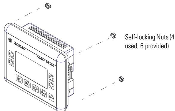
5. Alternately tighten the self-locking nuts until the terminal is held firmly against the panel.
