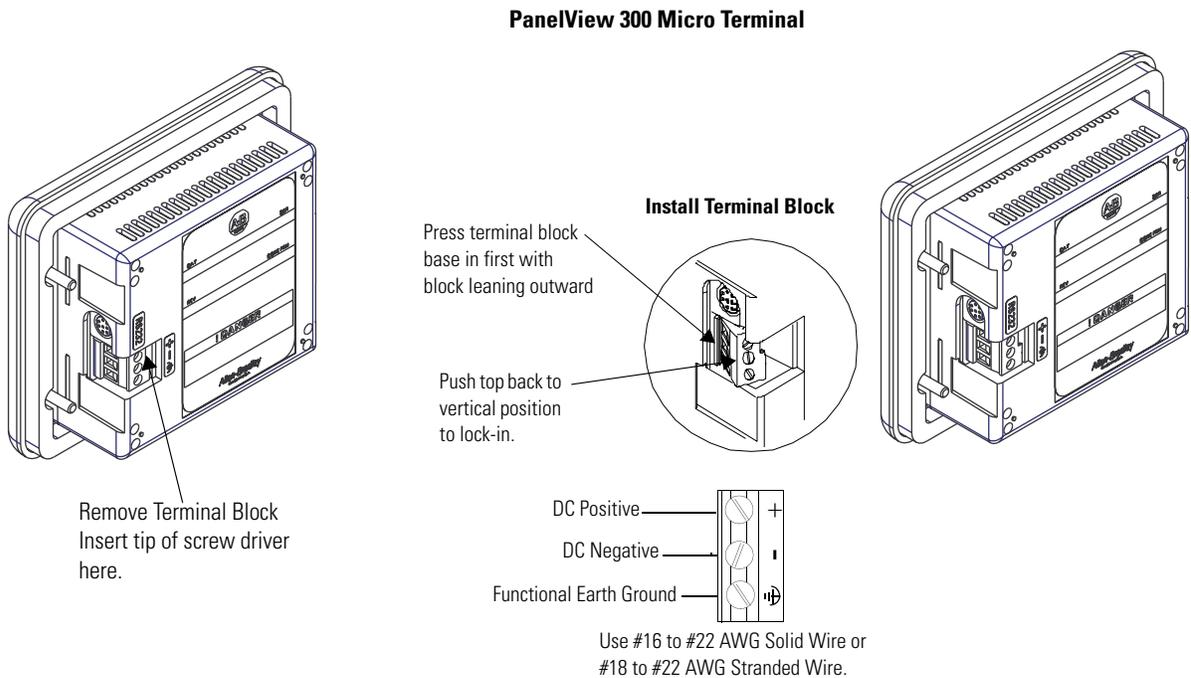
2. Secure the Functional Earth Ground (FE) wire to the correct terminal block screw.
