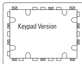
☒ = Recommended Placement of Mounting Clips
