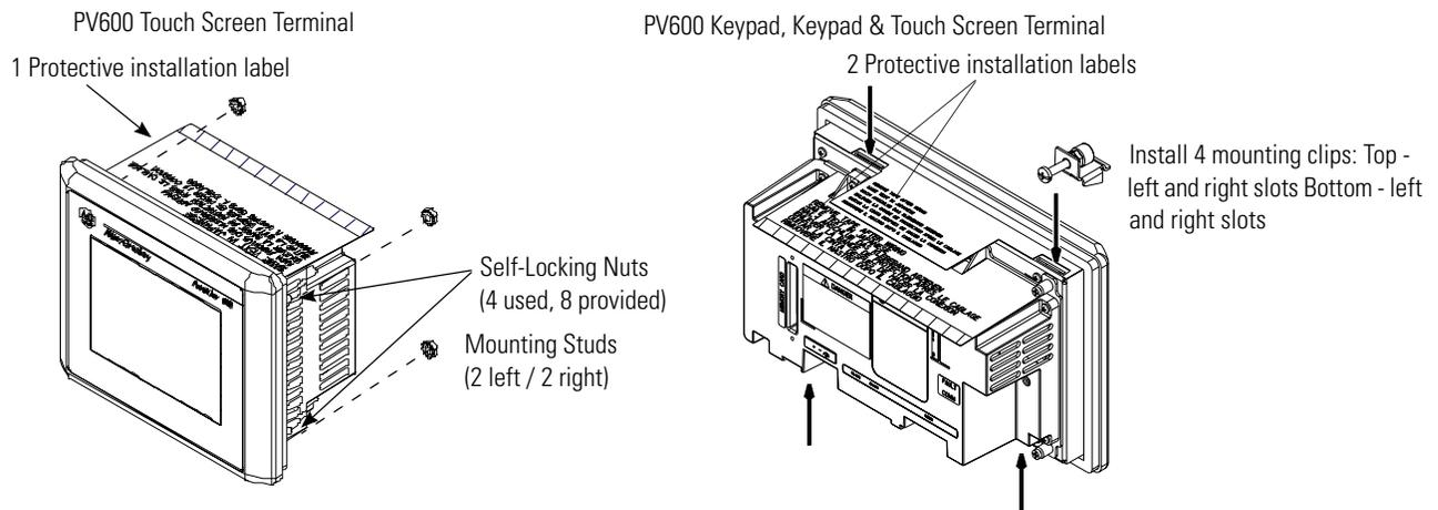
6. Alternately tighten the self-locking nuts or mounting clip screws until the terminal is held firmly against the panel.
