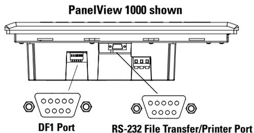
**Note:** The PanelView 300 has one DF1 port which is used for communication and transferring applications.
