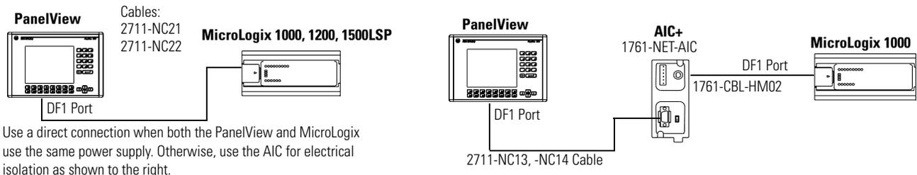
Use a direct connection when both the PanelView and MicroLogix use the same power supply. Otherwise, use the AIC for electrical isolation as shown to the right.
