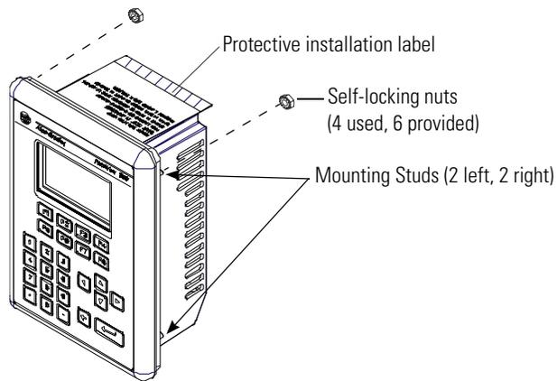
7. Alternately tighten the self-locking nuts until the terminal is held firmly against the panel
