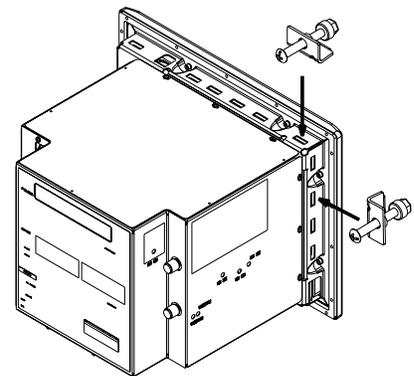
6. Alternately tighten the mounting clip screws until the terminal is held firmly against the panel.
