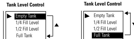
If the list contains more items than can appear at one time, the list scrolls. If the cursor is at the top or bottom of a scrolling list, the list scrolls one row at a time as the arrow keys are pressed.
