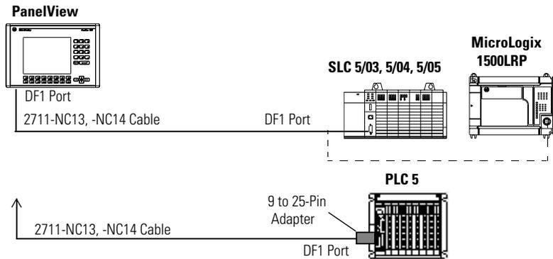
Use an optical isolator or equivalent when grounding level differences exist between the controller or modem and the PanelView.
