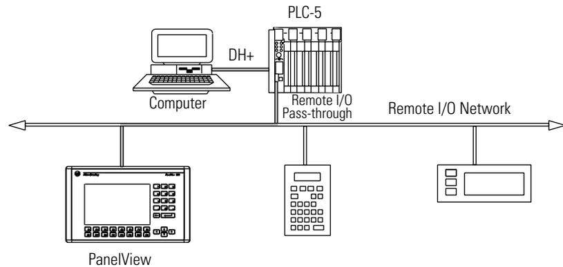
Follow these steps to transfer an application using remote I/O pass-through:
