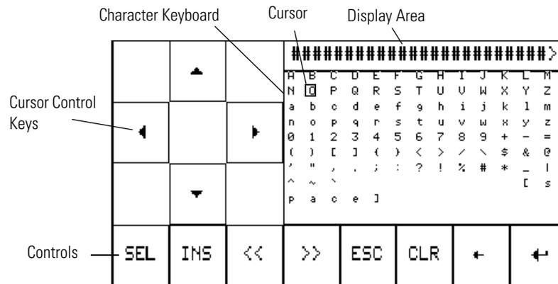
To select characters from the Character Keyboard, press the cursor control keys to move the cursor over a character and then press the SEL key. The character is entered in the Display Area. This area scrolls so you can enter a string that is longer than the Display Area. All characters are sent to the controller even if not visible.
