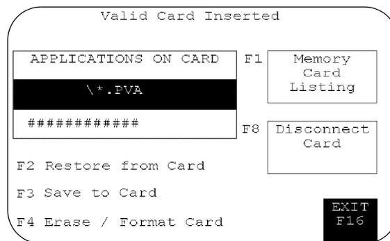
4. If necessary, press Erase/Format Card, [F4] key on keypad terminals, to format or erase a 2711-NM11, 2711-NM12, 2711-NM13, 2711-NM14, or 2711-NM15 memory card.
