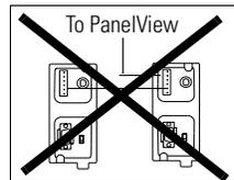
Do not connect the PanelView to Port 3 of the AIC+ when Port 3 is networked to other devices.
