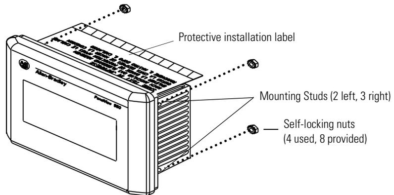
8. Alternately tighten the self-locking nuts until the terminal is held firmly against the panel.
