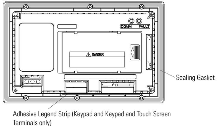
3. On the keypad and keypad and touch screen terminals, secure the ends of the legend strips to the legend strip adhesive.
