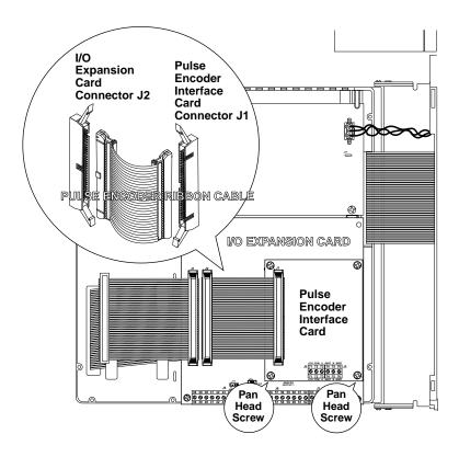
☐ 5 If an I/O Expansion Card is used, the Pulse Encoder Interface Card is mounted piggy back on the I/O Expansion Board and connected using hardware included with the Pulse Encoder Interface Kit.
