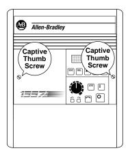
☐ 1 Remove and lock-out all incoming power to the drive. Loosen the (2) captive retaining screws and remove the drive cover.
