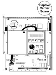
☐ 2 Loosen the captive carrier retaining screw and swing the carrier door open.
