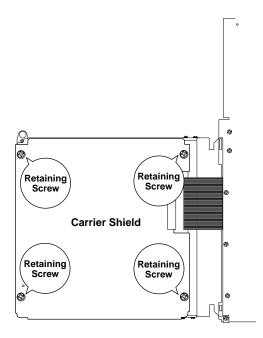
□ 3 To remove the carrier shield, remove the (4) retaining screws and unplug the ground wire at the Power Supply Board.
