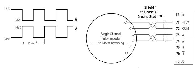
Belden 9728 or 9730 — (2) Conductor Twisted Shielded Cable Refer to the Cable and Wire Recommendations in the 1397 Use Manual for additional Wiring Specifications
