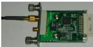
I. Insert it into SMB-75JWHD connector of electrical 155M interface board.
