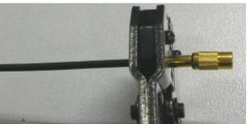
F. Place part of the tight loop into the suitable teeth hole (such as 151 marked) of the press line pliers to be tightly pressed. If there is no way to set outer bushing on the connector fitting, press it once more after the press line pliers is turned by 90 degrees.
