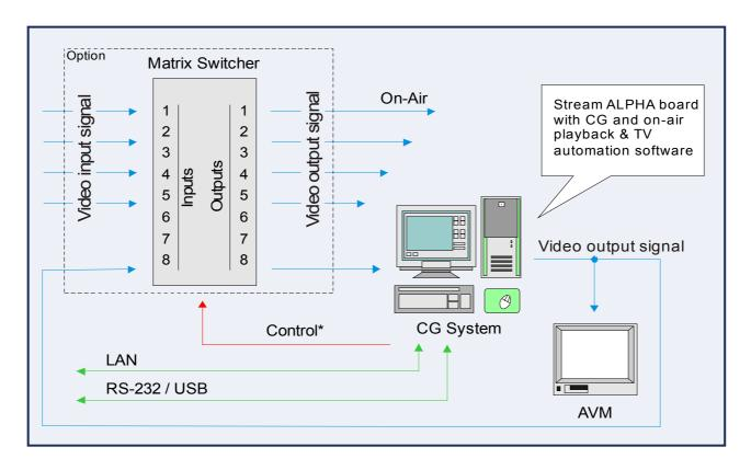
\*It is possible to control several external devices such as transcoder, mixer and switchboard.
