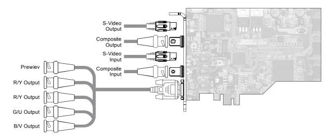
The connector cable is not included in the standard delivery set and can be purchased separately. The card default signal is RGB+Key; you can switch to YUV+Key mode by using the system settings (see below).
