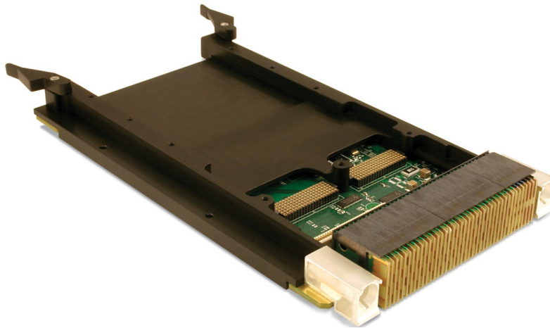
Figure 8. Innovative 3U VPX- XMC.3 adapter card (P/N 80260)
