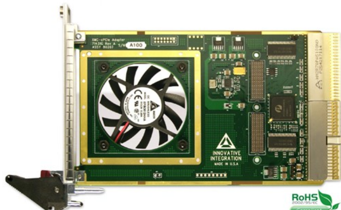
Figure 11. Innovative x8 Lane PCI Express – XMC.3 (8x lanes) adapter card (P/N 80173-0)
