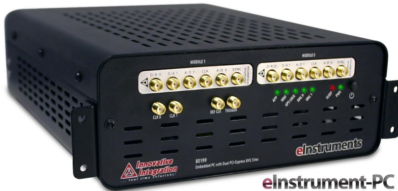
Figure 14. eInstrument PC – embedded PC (Windows/Linux) hosts two XMC modules (II P/N 90199)
