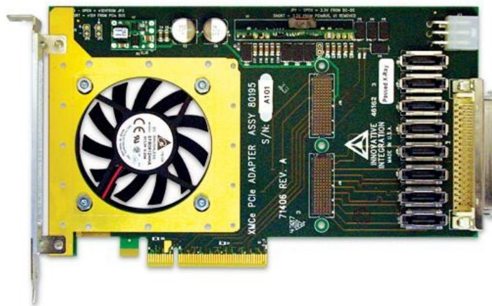
Figure 11. Innovative x8 Lane PCI Express – XMC.3 (8x lanes) adapter card (P/N 80173-0)
