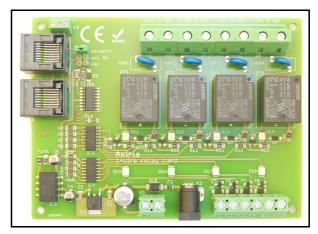
■ The 1-Wire slave chip can be powered parasitically, using an external 5 V line or using the on-board 5V supply.
