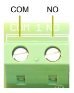
These connectors are wired to the contacts of the relays.
