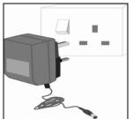
Attach the power supply cable to the connector on the rear of the balance. Plug the power supply module into the mains. The display will indicate the balance serial number (if set) and the software revision number followed by the capacity of the balance. Next the balance will run a self-test by displaying all segments and then will show zeros accompanied by the zero symbol. If the balance serial number is not set, the display will show dashes.
