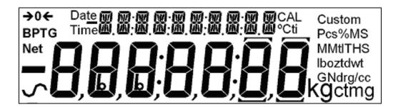
This display includes areas for the weight value (up to 7 digits), symbols for common weighing units, tare, stability, zero and low battery and a text area for menu.
