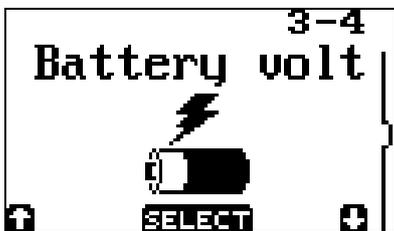
The battery voltage menu shows the current input voltage of the battery.
