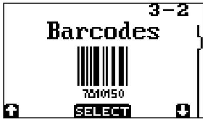
The barcode menu enables or disables barcode types that are supported by the OPL9728. More barcodes can be enabled at the same time.
