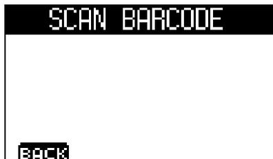
Barcode can now be scanned by pressing the trigger button. Keyboard input is also possible. To enter alpha data press the shift button and while keeping it pressed press any of the numeric keys. To enter the input data press the ENT key.
