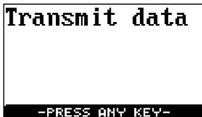
When the transmit data message appears on the display put the OPL9728 in the cradle and then press a key. On the PC needs to run an application to receive the database.
