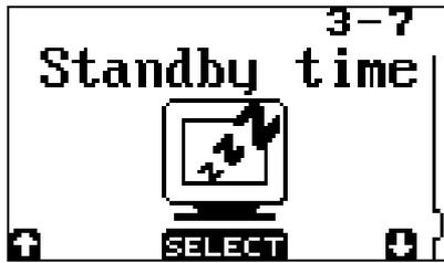
Selecting the standby time sets the time the terminal stays on when no key is pressed. When pressing one of the three keys will turn the terminal back on.
