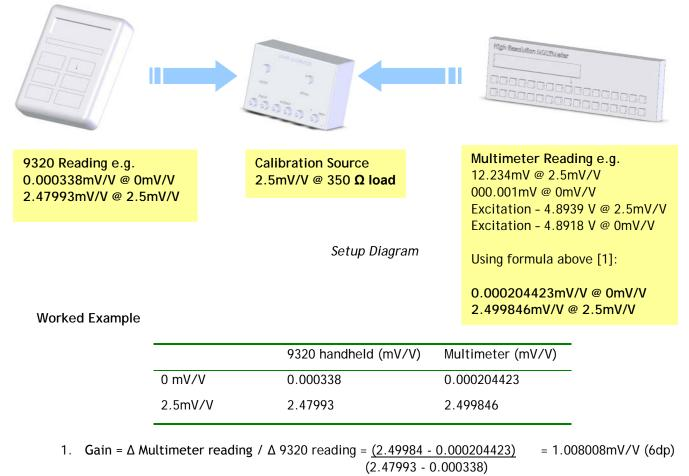
2. Offset = Multimeter reading - 9320 reading = 0.000204423 - 0.000338 = - 0.000096mV/V (6dp)
