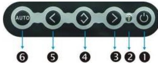
❶ **POWER SWITCH:** Pushing the power switch will turn the monitor on. Pushing it again to turn the monitor off.
