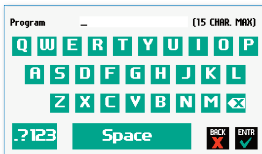
New Program Name Entry screen showing letter keys. To view numbers/symbols, choose the ?123 use button in the lower left corner
